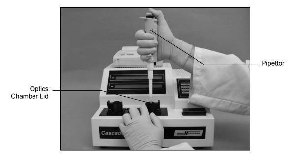
Fig. 6-2. Simultaneously Press Optics Chamber Lid and Pipette Reagent
